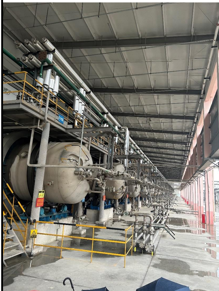
Figure 2: Insoluble sulphur production facilities. In each tank, key chemicals (sulphur, carbon disulfide) are automatically rotated continuously as part of the manufacturing process
